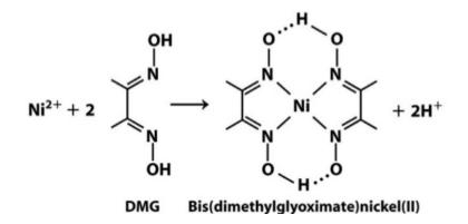
The reaction is performed in a solution buffered by an ammonia buffer to avoid falling in pH value below 5. If the pH becomes too low the equilibrium of the above reaction favours the formation of the nickel(II) ion, causing the dissolution of DMG-Ni complex.
